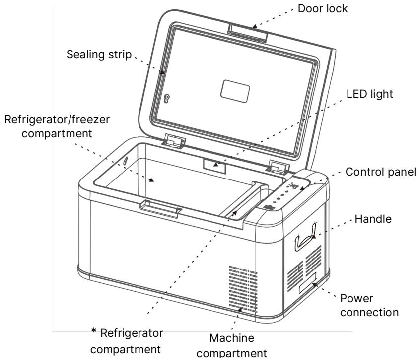
\* The temperature of the small compartment changes along with the large compartment. Only the large compartment can be adjusted, while the small compartment is typically used as a refrigerator to keep food from freezing.
